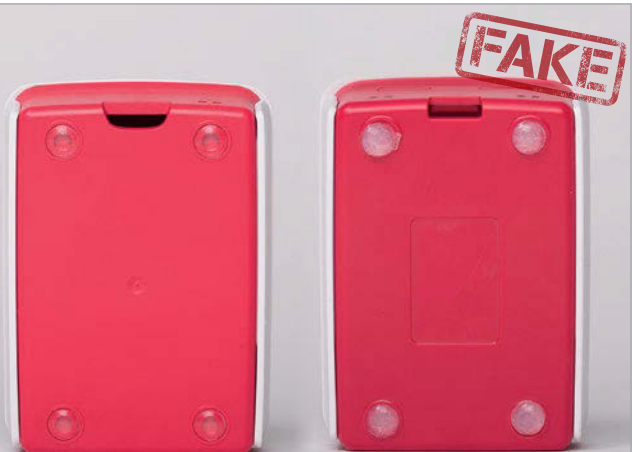
Above This fake case has two sets of light pipes Below The shoddy feet on this case are a clear sign of a fake
