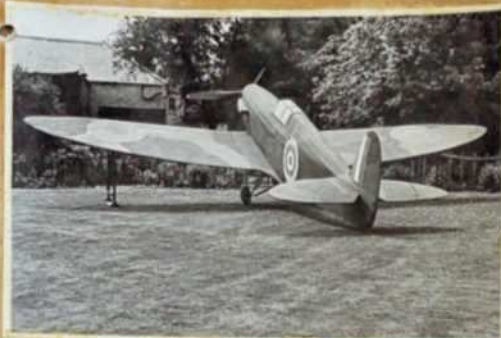
THREE DIMENSIONAL SPITFIRE In this case built on old Moth's undercarriage
