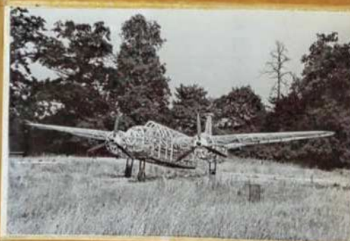
THREE DIMENSIONAL DUMMY BOSTON SHOWING CONSTRUCTION
