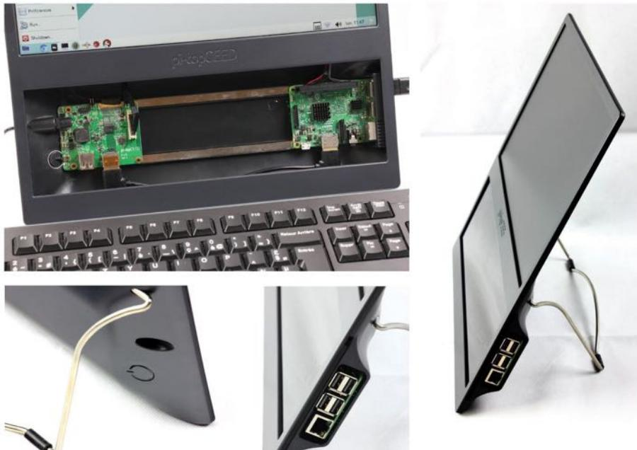
LES RAILS MÉTALLIQUES DERRIÈRE LA TRAPPE AMOVIBLE PERMETTENT DE PLACER D'AUTRES MODULES, MAIS SURTOUT LE RASPBERRY PI. LES AIMANTS SONT TRÈS PUISSANTS ET L'OUVERTURE SUR LE CÔTÉ PERMET D'AVOIR ACCÈS AUX PORTS USB ET RJ45. L'UNIQUE ALIMENTATION (POUR L'ÉCRAN ET LE RASPBERRY) N'EST PAS MICRO-USB, MAIS AU FORMAT JACK 5 MM. LE BOUTON DE MISE EN MARCHE EST UN PEU RAIDE PAR CONTRE LA TIGE EN MÉTAL AU DOS PERMET D'INCLINER LE PI-TOP Ceed SUR 65°.
