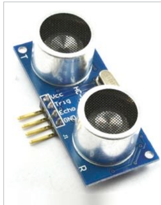
Left The HC-SR04 Ultrasonic Rangefinder. Cheap-as-chips sonar
